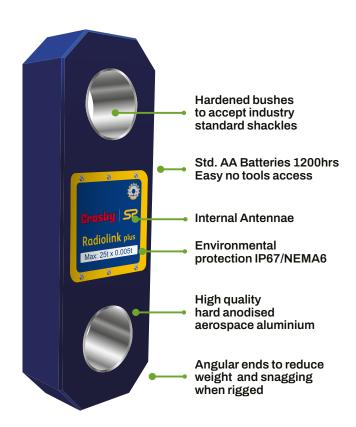
Crosby Straightpoint Radiolink Plus is designed to be rigged with Crosby standard shackles - DNV-GL type approved wireless tension load cell capable of weighing and dynamic load monitoring in capacities from 1t to 300t - from stock with an ATEX and IECEx version available for hazardous areas, zones 0, 1 & 2.
